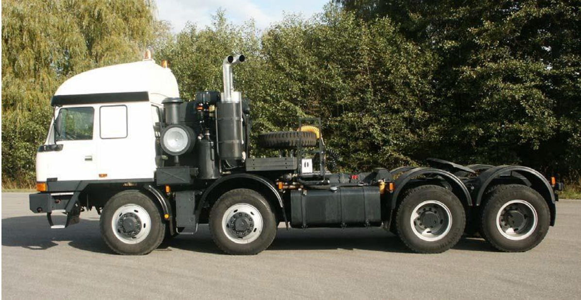
FIGURE 2.5: Israeli MOD (IMODHETT) 8X8 TATRA equipped with Single-Fluid-Forward®, and Twin Disc Model 3600 transmission. The SFF reservoir is visible located ahead the #2L wheel behind the air cleaner. The TATRA IMODHETT successfully completed first article testing in Israel in 2006.
