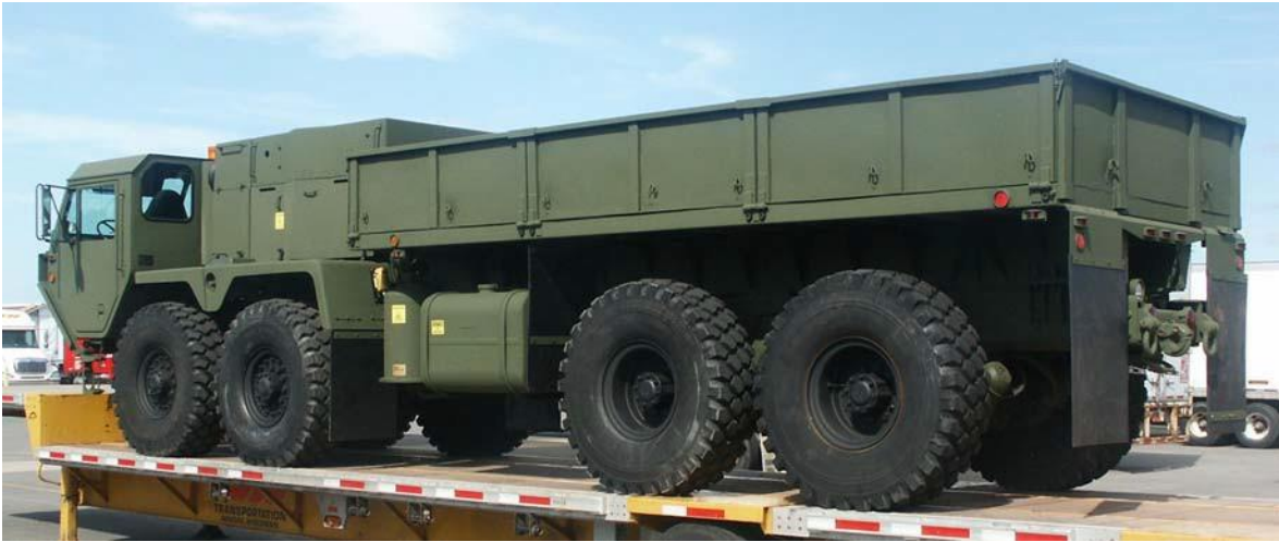
FIGURE 2.1: ISLAND CITY 8X8 HEMTT Upgrade (HEMTT+) Advanced Technical Demonstrator equipped with Single-Fluid-Forward®, Twin Disc Model TD61-1179 transmission, CUMMINS 565 hp ISX engine and numerous upgrades presented by ADI Technologies at the 2006 Platform Systems Demonstration (PSD) at Aberdeen Proving Grounds (APG). The SFF Reservoir is located behind the left fender. The HEMTT+® was developed and assembled by ISLAND CITY, LLC. Twin Disc Corporation uses the HEMTT+® to develop and test advanced defense transmission systems.
