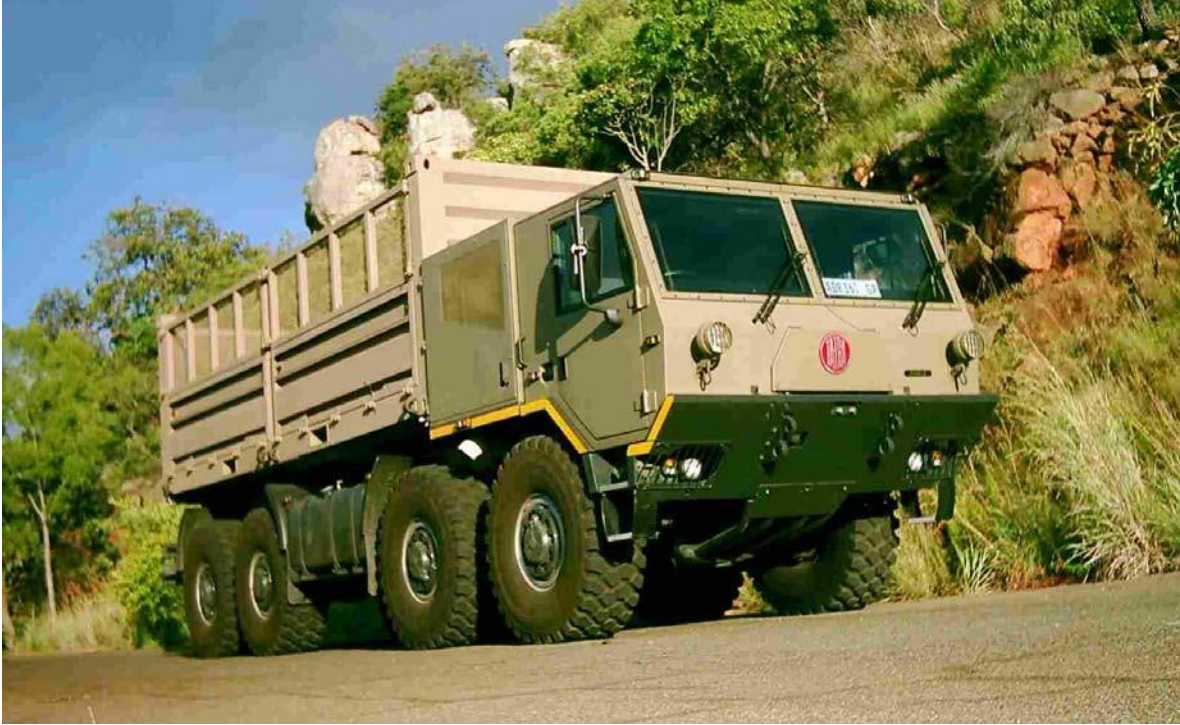
FIGURE 2.3: South Africa MOD 8X8 (SA8X8) TATRA equipped with Single-Fluid-Forward®, and Twin Disc Model TD61-1179 transmission. The rectangular SFF reservoir is not visible - located in the center compartment. The TATRA SA8X8 successfully completed first article testing in South Africa in 2005.
