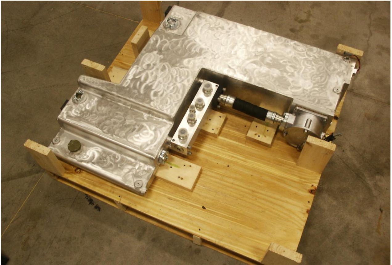
FIGURE 2.10: USMC MPC SFF hydraulic reservoir.
