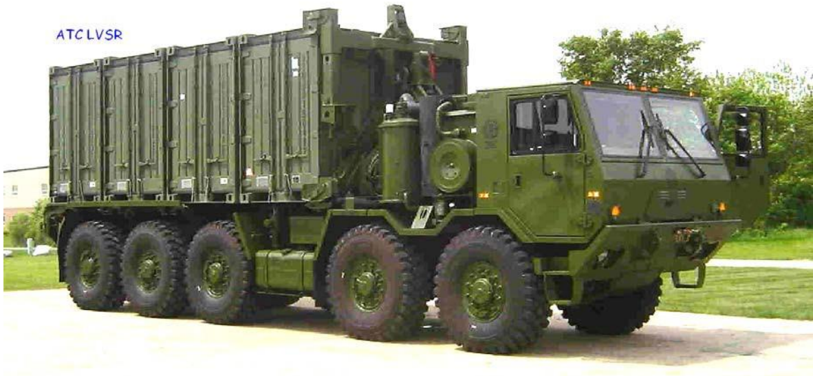
FIGURE 2.2: USMC LVSR 10X10 (ATC/TEREX LVSR) American Truck Company/TEREX equipped with Single-Fluid-Forward®, Twin Disc Model TD61-1187 Transmission and 625 hp C18 Caterpillar engine. The SFF reservoir is visible, located above the #2R fender. The ATC/TEREX LVSR successfully completed first article testing at APG in 2005/2006.
