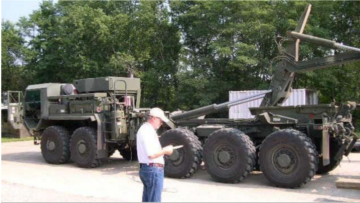
FIGURE 2.0: USMC 10X10 LVSR Technical Demonstrator (LVSR TD) equipped with Single-Fluid-Forward®, Twin Disc TD61-1183 transmission and Detroit 600 hp 60 Series engine undergoing testing at Quantico, VA. The SFF reservoir is visible behind the left fender. The LVSR TD was developed and assembled at the Nevada Automotive Test Center (NATC). Island City, LLC provided the principle integration engineering for the LVSR TD. The LVSR TD has undergone extensive performance and endurance testing at the NATC proving grounds. The USMC used the LVSR TD to evaluate and form the technical requirements for the LVSR program.
