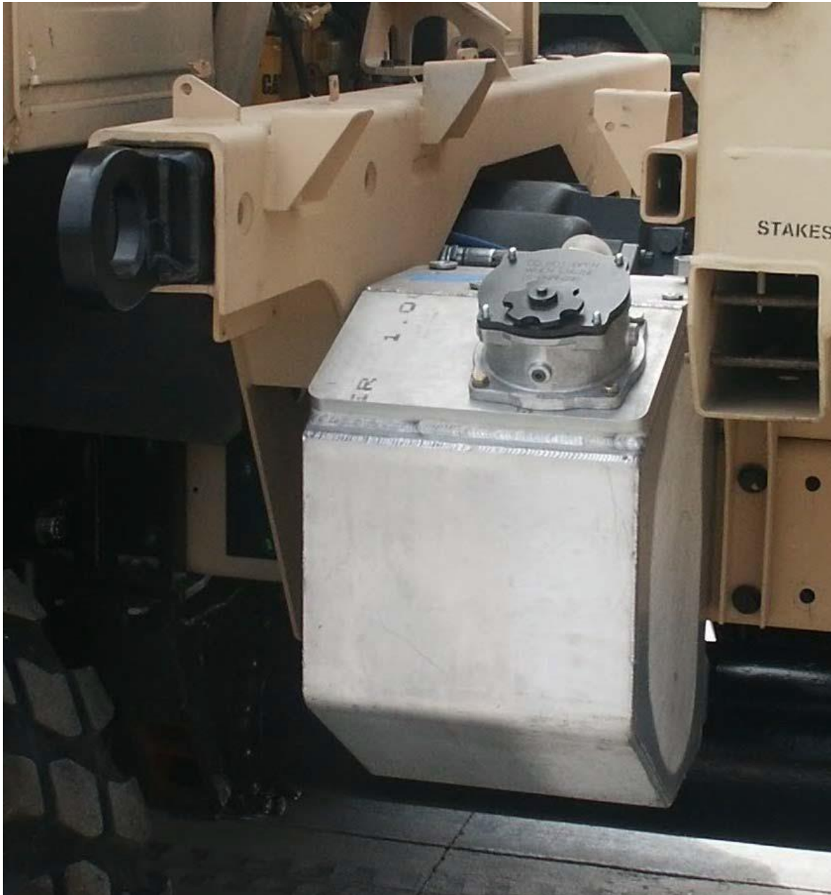
FIGURE 2.8: FMTV+ SFF reservoir located on the drivers' side behind the forward hard lift support. The reservoir is equipped with a capacitance fluid level, and indirect visual fluid level site gage.
