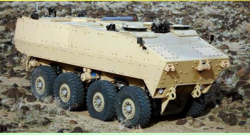
USMC <u>MPC Technical Demonstrator</u> 22-1/2 ton equipped with *Single-Fluid-Forward*® undergoing testing at NATC. Exclusive Common-Hydraulic-System technology and integration engineering from ISLAND CITY, LLC.
